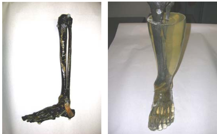
Figure E.16: The Frangible Synthetic Lower Leg (FSL), Without (left) and With (right) Gelatine.
