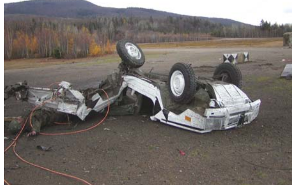
Light Logistic Vehicle – After the test
