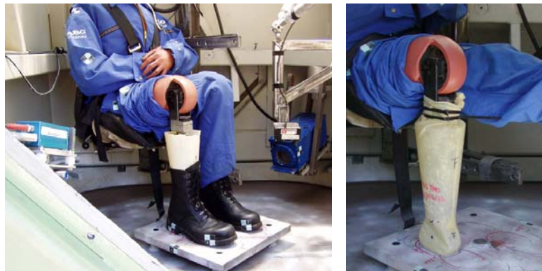
Figure E.19: TROSS Tests on the CLL With (left) and Without (right) Boot (Pictures courtesy of TNO).
