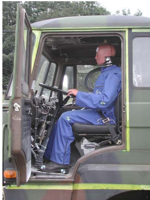
Figure 4.4: Hybrid III ATD in a Truck before the Mine Test.
