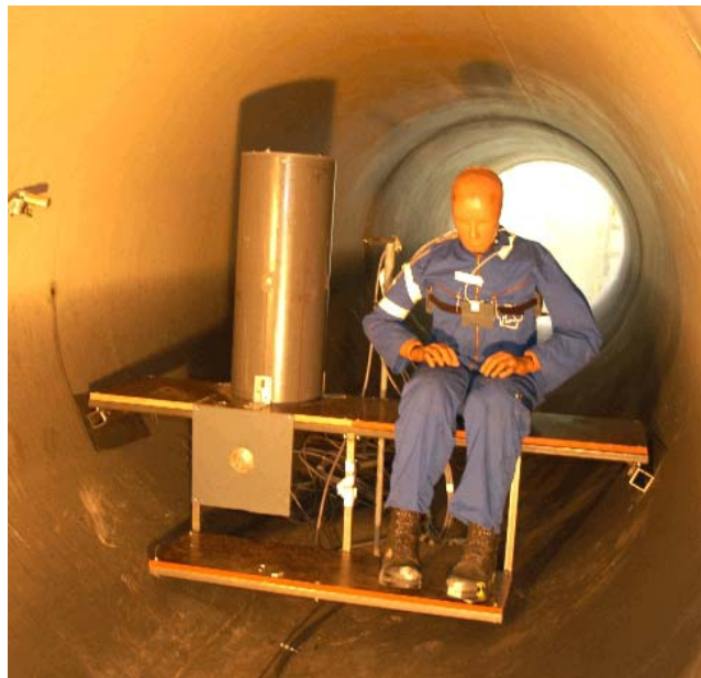
Figure 4.7: BTM (left) and Hybrid III ATD (right) in Blast Tunnel [Horst, 2005].
