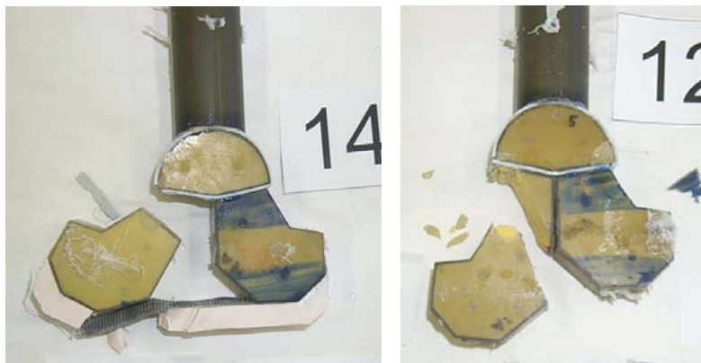
Figure E.20: Results of Laboratory Axial Tests on the CLL With (left) and Without (right) Boot [Manseau, 2005b].
