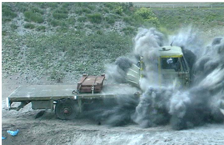
Figure 1.1: Example of Mine Detonation under a Logistic Vehicle.
