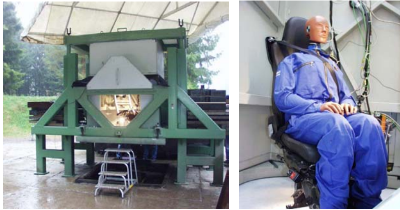
Figure E.17: Exterior (left) and Interior (right) View of TROSS™ Set-up (Pictures courtesy of IABG).
